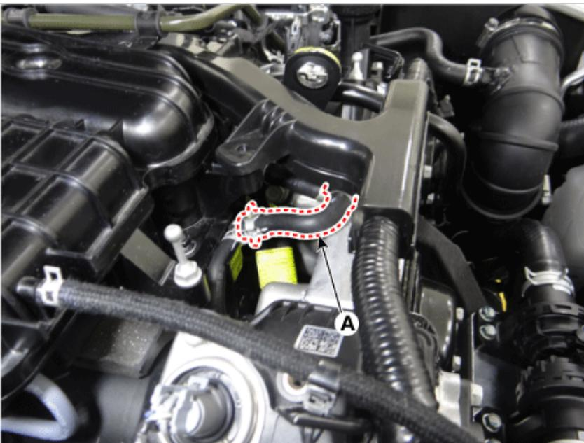
12. Fill with fluid mixture of coolant and water (55 - 60% / or 45 - 50% in North America, Europe and China) slowly through the radiator cap.
