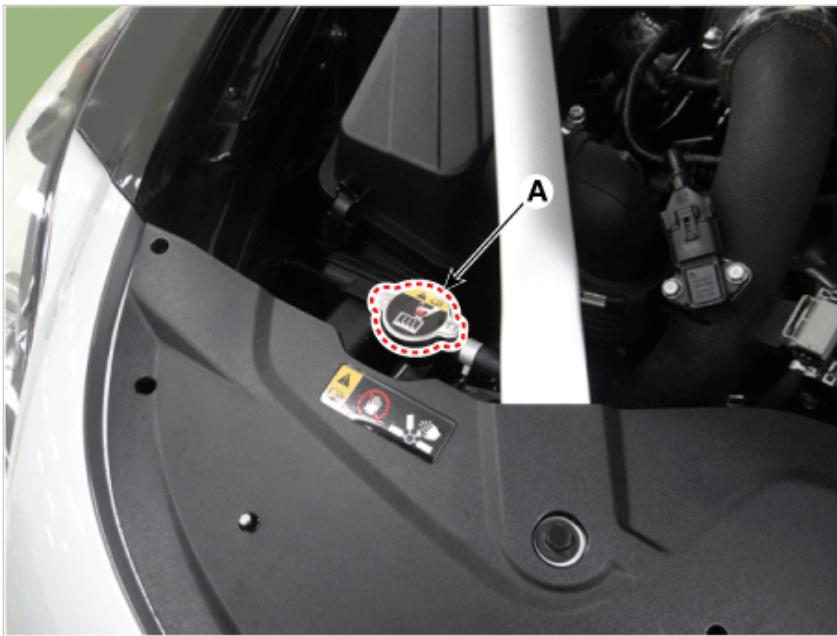
29. Check the coolant level and then fill the reservoir tank to the "F" line with coolant.
