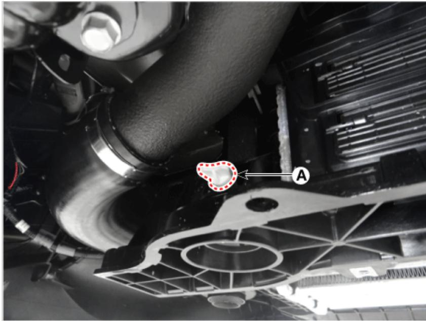
5. Tighten the radiator drain plug securely.
