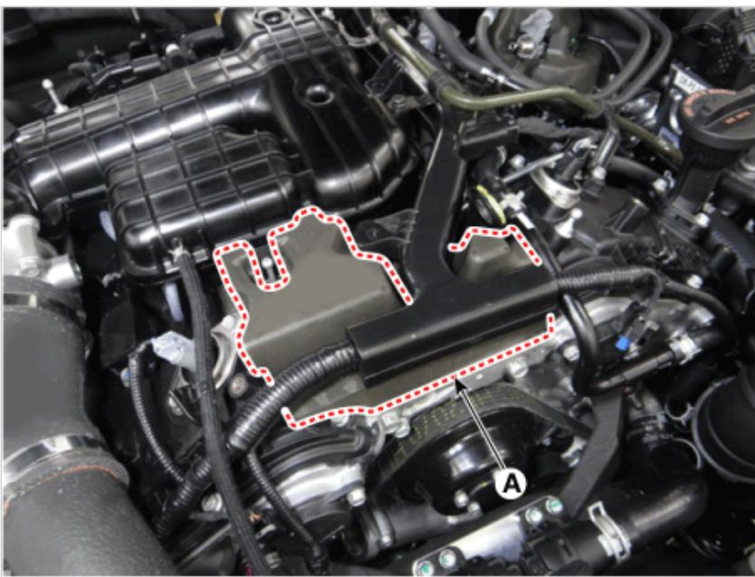
11. Disconnect the coolant vent hose (A).
