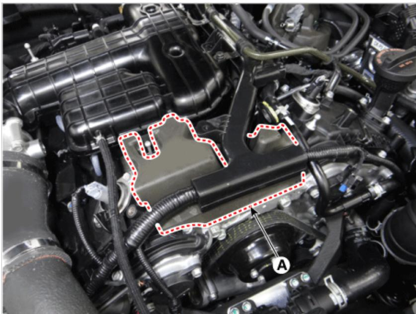
31. Install the wiring protector (A).
